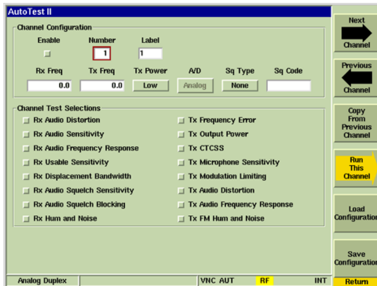
Fig. 8-50 Channel Configuration Tile
