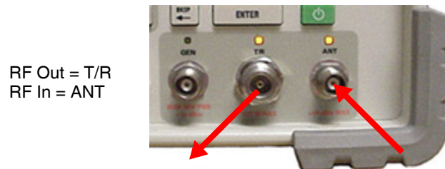
Fig. 3-27 TR/ANT Two Port Duplex Test Setup
