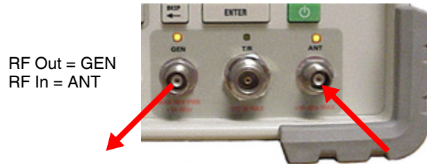
Fig. 3-25 GEN/ANT Two Port Duplex Test Setup
